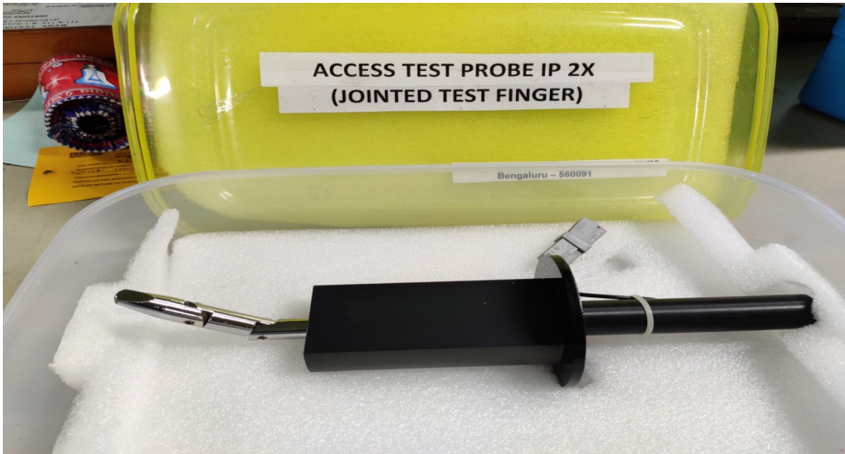
Name of Instrument : IP 2X Test probe Jointed Test Finger for Degree of Protection Uses : Testing of LED lamp, CFL, LED street light, LED floodlight, LED Luminaries
