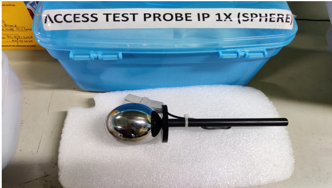
Name of Instrument : IP 1X Test probe(S phere) for Degree of Protection Uses : Testing of LED lamp, CFL, LED street light, LED floodlight, LED Luminaries
