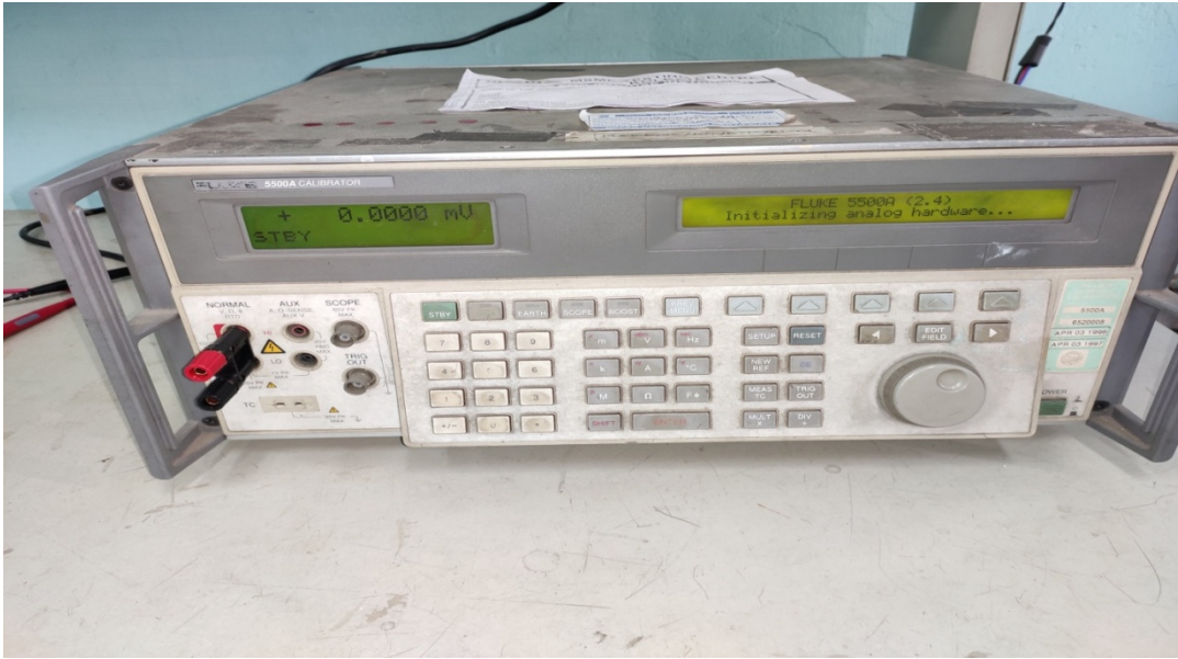
Name of Instrument: Multi Product Calibrator, Fluke, USA Uses : Calibration of AC/DC Voltage, AC/DC Current , Frequency, Capacitance etc.
