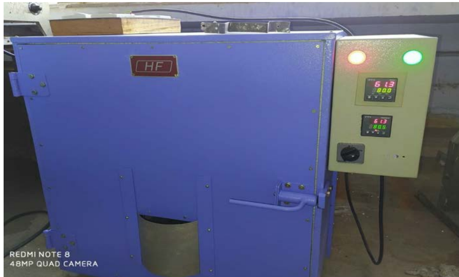
Name of Instrument : Electric Oven to check LED Gears and Drives Uses : Testing of LED Gears and Drives of LED luminaire as per IS 15885 (Part 1): 2011
