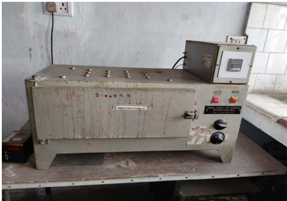
Name of Instrument : Thermal Stability Test Apparatus Uses : Testing Cables as per IS 694 & IS 7098
