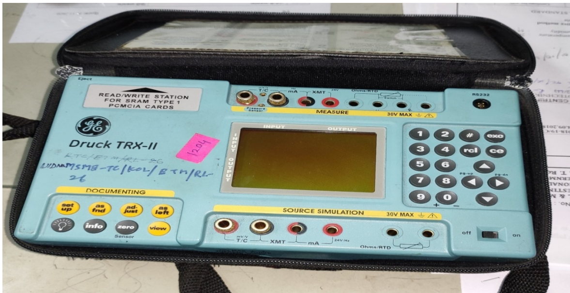
Name of Instrument :Multifunction calibrator, Make Druck Uses : Calibration of Temperature indicator with sensor
