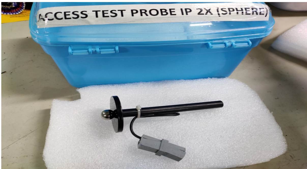
Name of Instrument : IP 2X Test probe Sphere for Degree of Protection Uses : Testing of LED lamp, CFL, LED street light, LED floodlight, LED Luminaries
