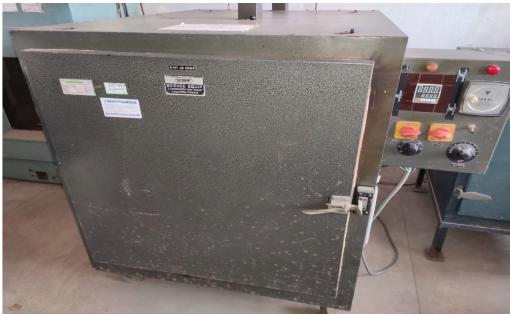
Name of Instrument :Ageing Air Oven Uses : Testing of GLS Lamp as per IS 418 -2004
