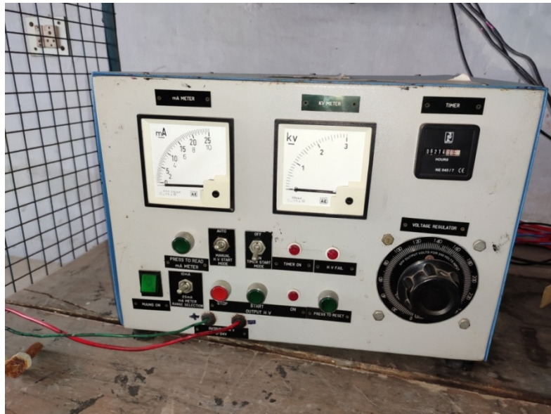
Name of Instrument : Hot Set Apparatus Uses : Testing Cables as per IS 694 & IS 7098
