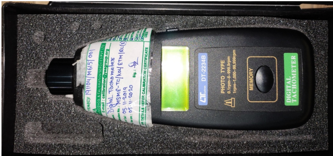
Digital Tachometer Uses : Measurement of Fan RPM
