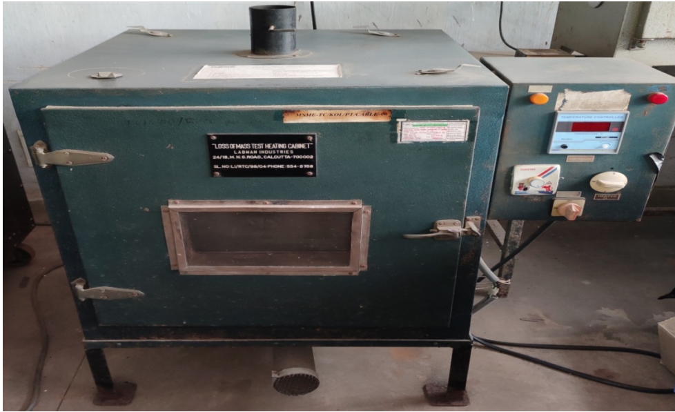
Name of Instrument : Loss of Mass Test Heating Cabinet Uses : Testing Cables as per IS 694 & IS 7098
