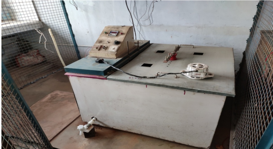
Name of Instrument : Water Bath Uses : Testing Cables as per IS 694 & IS 7098
